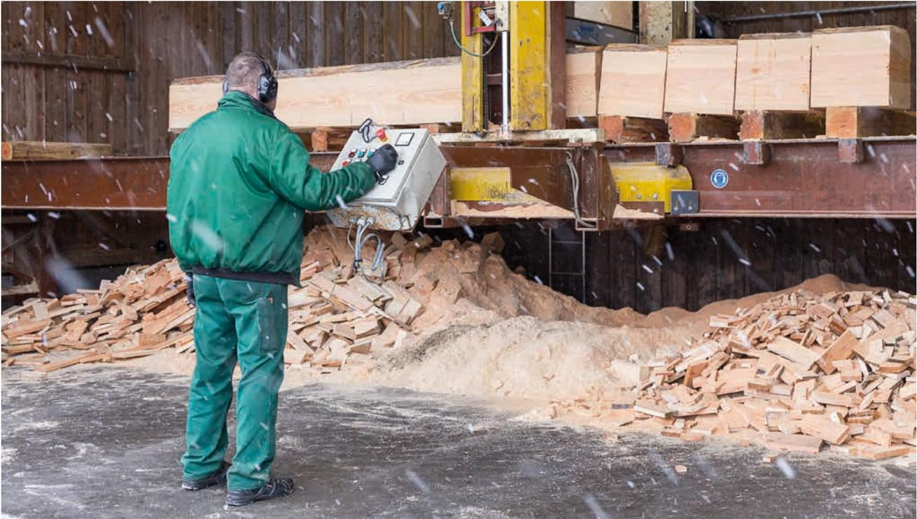
▲ A large oak log is cut into blocks on one of the sawmill's large saws.
