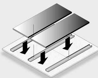
**Figure 2:** Acoustic Pads for Troldtekt Elements placed loosely between the C60 profiles.
