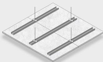
**Figure 1:** Troldtekt Elements suspended ceiling installed.
