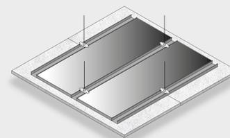
**Figure 3:** Acoustic Pads for Troldtekt Elements installed.
